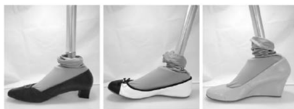
Fig 1. A Prosthetic foot aligned for One Particular Heel Rise (Left) is inherently misaligned when wearing shoes of other Heel Rises, As Demonstrated by The angle of the respective Pylons (Center, Right).
