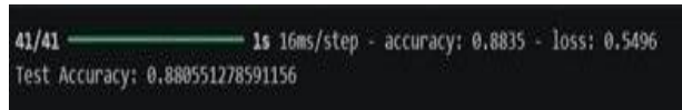
Fig. 5: MobileNetV2 final evaluation: test accuracy 88.06%, test loss 0.5496. Inference is 5.3x slower (16ms/step vs. 3ms/step for the custom CNN).
