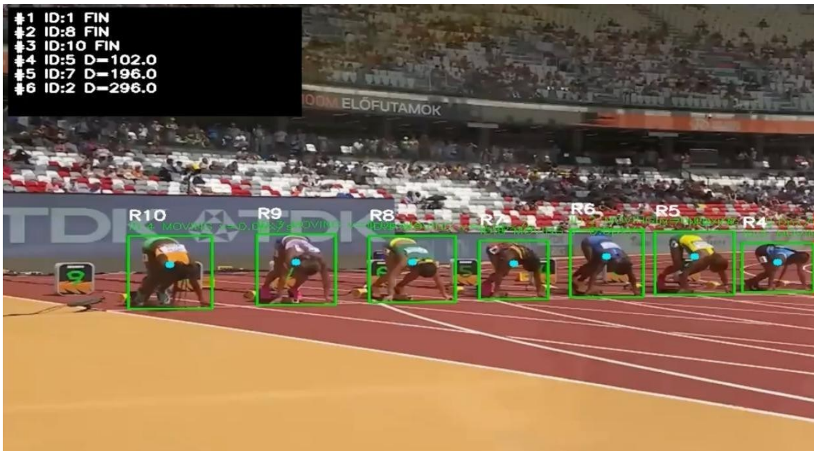
Figure 3: Pre-race start block detection. All runners in set position with bounding boxes (R4–R10), unique IDs, and MOVING state – confirming successful pre-race tracking initialisation.
